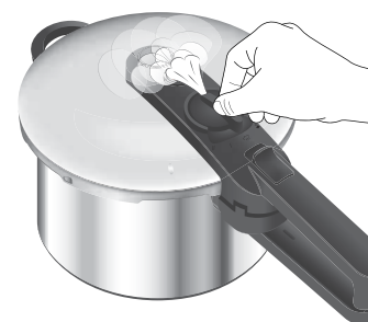
Abb. 17: Fast pressure release
