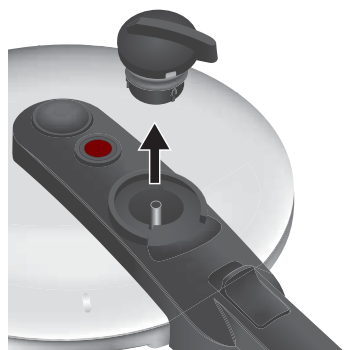
Abb. 21: Detaching the pressure regulator
